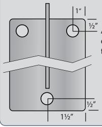
All holes are measured from edge of bracket or bend to the center of the hole.
